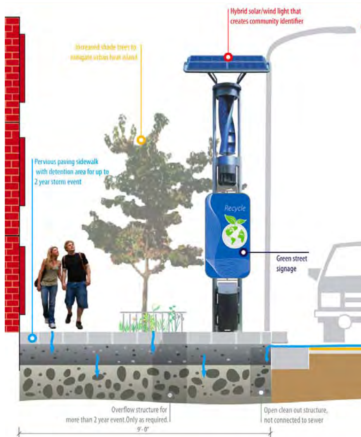
Chicago, IN: Eye-catching solar and wind-powered light and signage.
