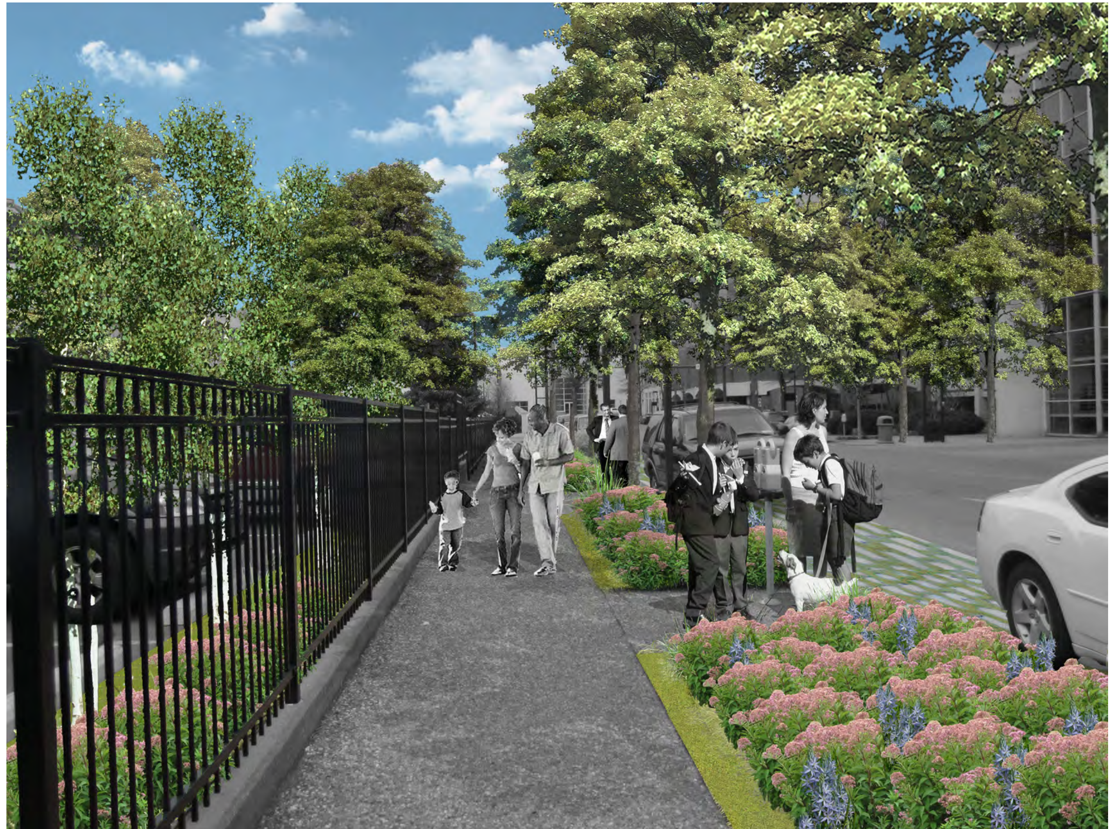
PROPOSED BIORETENTION BASIN + POROUS PAVING PARKING LANE + GREENING OF SURFACE PARKING
