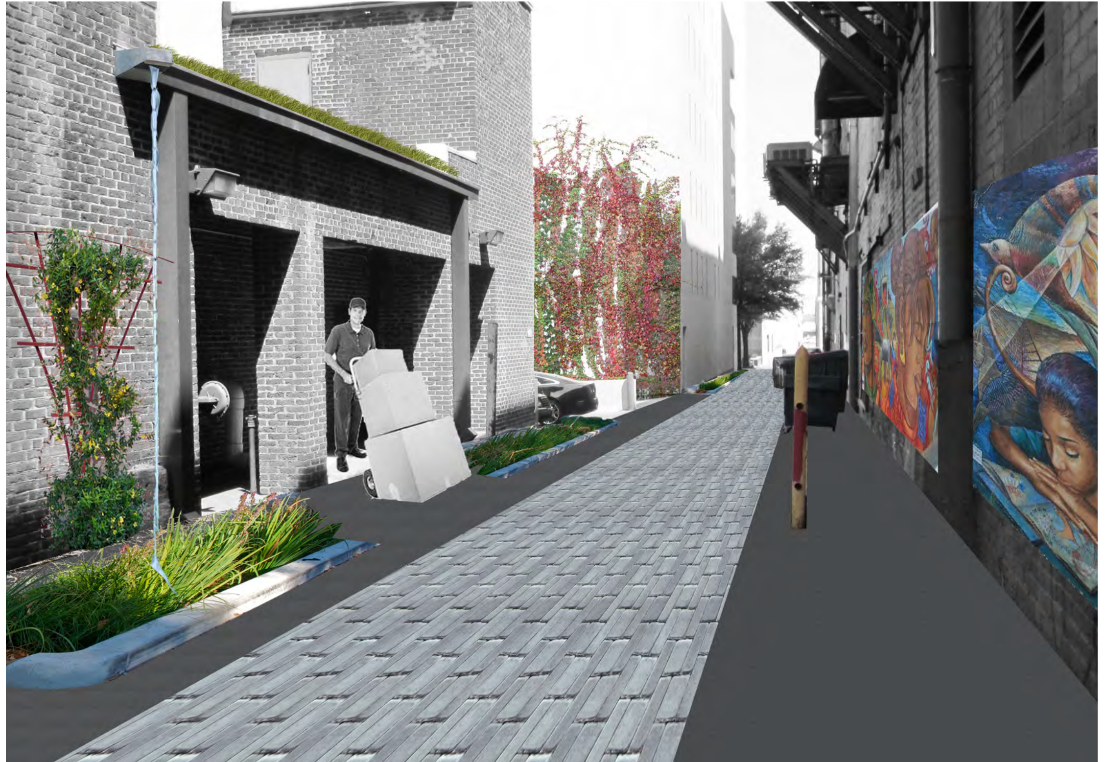
PROPOSED GREEN ALLEY (BIO-RETENTION BASIN + GREEN ROOF + DOWNSPOUT + POROUS PAVERS + MURAL)
