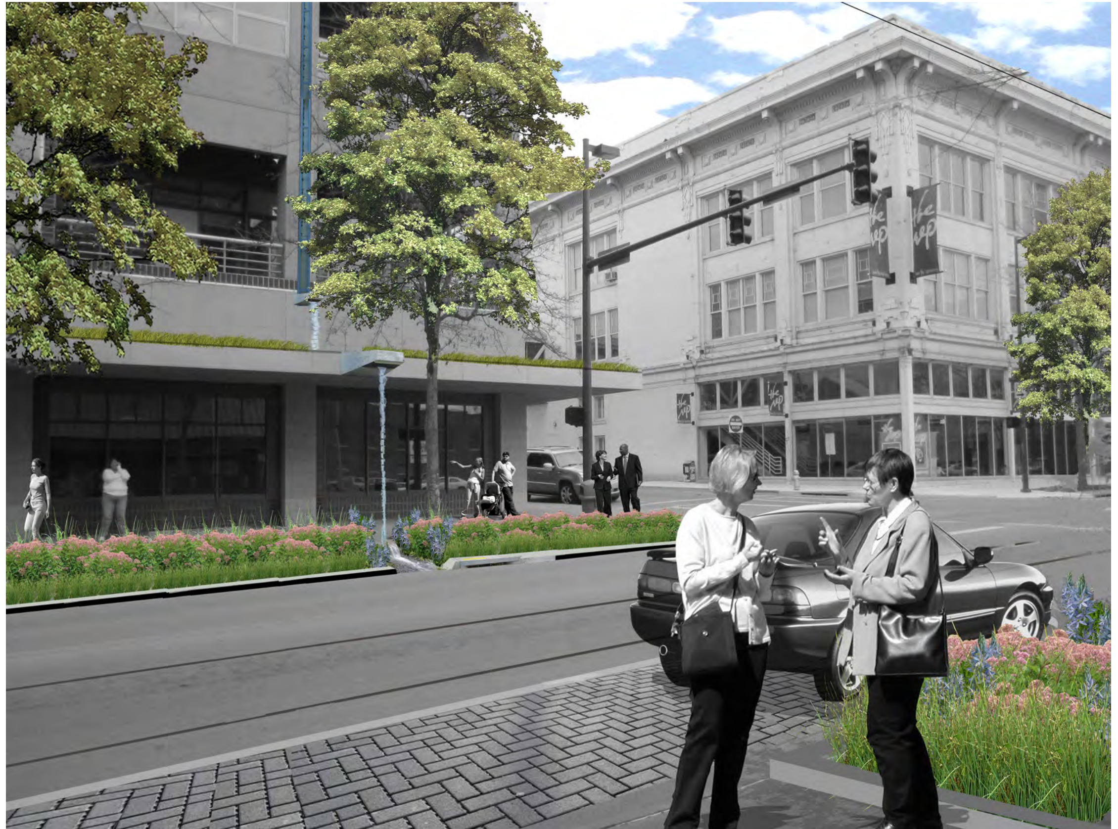
PROPOSED BIORETENTION BASIN + PORUS PAVING PARKING LANE + DOWNSPOUT RAIN GARDEN + TROLLEY TRACK
